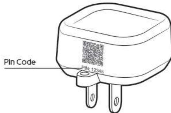
The DSK is printed on the Range Extender 7 itself located right under the QR code.
