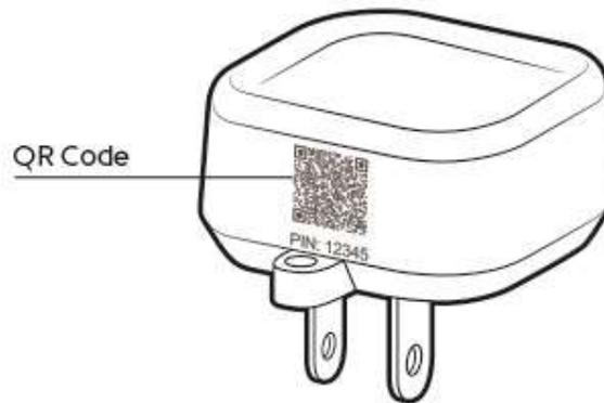
4. Within 10 minutes after powering your Range Extender 7, it will automatically get included into your Z-Wave gateway/controller/hub.
