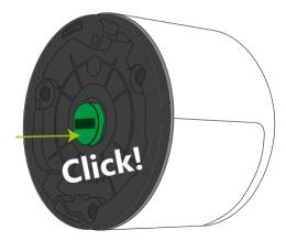
**8. Fit the tailpiece to the middle of the housing base** Fit the Danalock over the back plate. Make sure the tailpiece hits the slide in the middle of the adapter.
