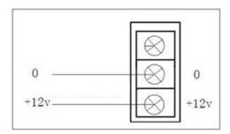
**Step 1:** Separate Panel and Bottom case by removing the screw at the bottom of device. Insert all wires into the right terminals and tighten screws. The wiring diagram is shown above.
